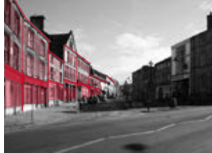
Moor Lane, looking east: 2 - 3 storey Georgian townhouses, 2 - 3 bays wide. Strong horizontal line of ground floor shop fronts (Victorian or later).
