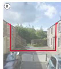
Shaw Street towards footbridge: 6m carriageway, 1.5m pavements.
